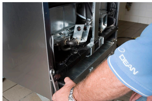
Figure 2 Pry on the loosened manifold as necessary on two-vat units to install the inward pointing elbow.
