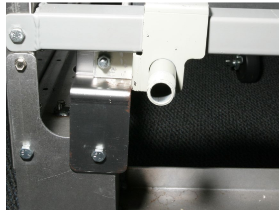
Figure 7: The rear-discharge plumbing is mounted as shown above on three and four-vat fryers.
